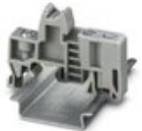
End clamp, width: 9.5 mm, height: 35.3 mm, material: PA, length: 50.5 mm, Mounting on a DIN rail NS 32 or NS 35, color: gray
