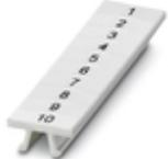
Zack marker strip, Strip, white, labeled, Printed vertically: consecutive numbers 1 ... 10, 11 ... 20, etc. up to 91 ... 100, mounting type: snap into tall marker groove, for terminal block width: 4.2 mm, lettering field size: 4.2 x 10.5 mm, Number of individual labels: 10
