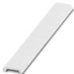
Zack Marker strip, flat, can be ordered: Strip, white, labeled according to customer specifications, mounting type: snap into flat marker groove, for terminal block width: 4.2 mm, lettering field size: 4.2 x 5.2 mm, Number of individual labels: 10
