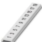
Zack Marker strip, flat, Strip, white, labeled, printed horizontally: Odd numbers 1 - 19, 21 - 39, etc. up to 81 - 99, mounting type: snap into flat marker groove, for terminal block width: 4 mm, lettering field size: 5.15 x 4.15 mm, Number of individual labels: 10
