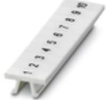
Zack marker strip, Strip, white, labeled, printed horizontally: consecutive numbers 1 ... 10, 11 ... 20, etc. up to 91 ... 100, for terminal block width: 4.2 mm, lettering field size: 4.2 x 10.5 mm, Number of individual labels: 10
