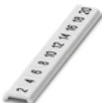
Zack Marker strip, flat, Strip, white, labeled, printed horizontally: consecutive numbers 2 ... 20, 22 ... 40, etc. up to 82 ... 100, mounting type: snap into flat marker groove, for terminal block width: 4 mm, lettering field size: 5.15 x 4.15 mm, Number of individual labels: 10
