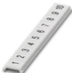
Zack Marker strip, flat, Strip, white, labeled, printed horizontally: consecutive numbers 1 ... 10, 11 ... 20, etc. up to 91 ... 100, mounting type: snap into flat marker groove, for terminal block width: 4 mm, lettering field size: 4.2 x 5.2 mm, Number of individual labels: 10
