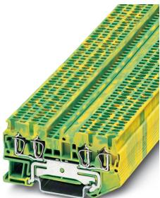
Ground modular terminal block, connection method: Spring-cage connection, number of connections: 4, cross section: 0.08 mm<sup>2</sup> - 1.5 mm<sup>2</sup>, AWG: 28 - 16, width: 4.2 mm, color: green-yellow, mounting type: NS 35/7,5, NS 35/15
